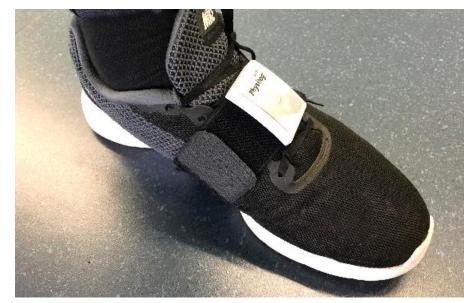
Fig. 1: foot-worn inertial sensor
