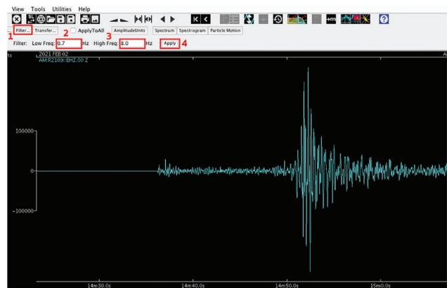
Fig. 7: Illustration for filtering data.
