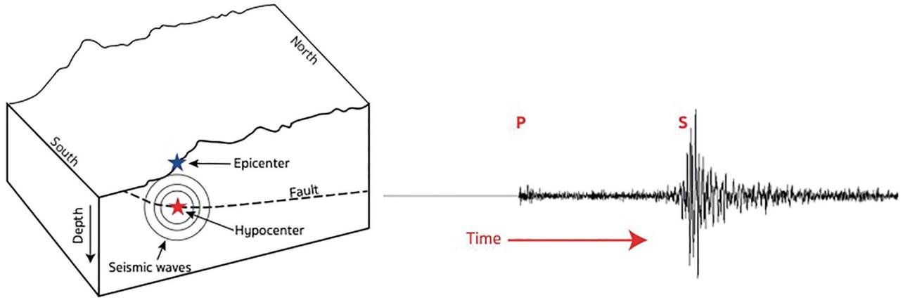
**Fig. 1:** Pictorial representation of some basic terminology used here. Schematic illustration of earthquake’s epicenter and hypocenter (Left). Example of earthquake recorded with P and S body waves clearly seen (Right).
