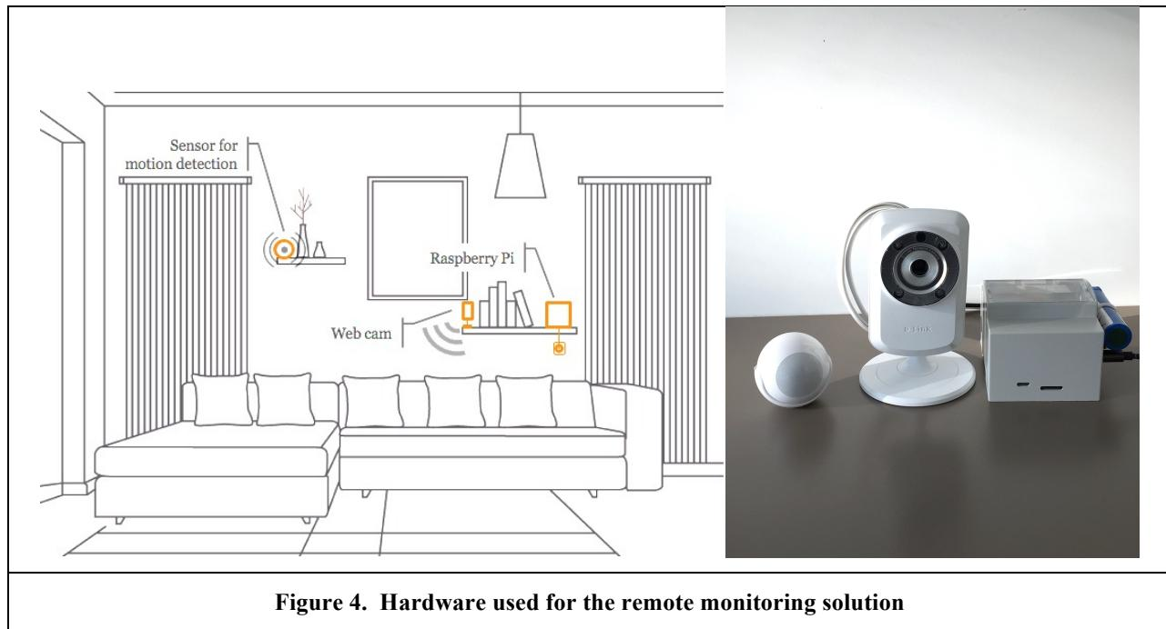
Figure 4. Hardware used for the remote monitoring solution
