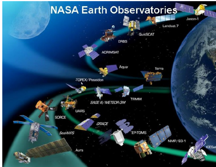
Figure 164: The Earth Observing System is a coordinated series of polar-orbiting and low inclination satellites for long-term global observations of the land, surface, biosphere, solid Earth, atmospheres and oceans.
