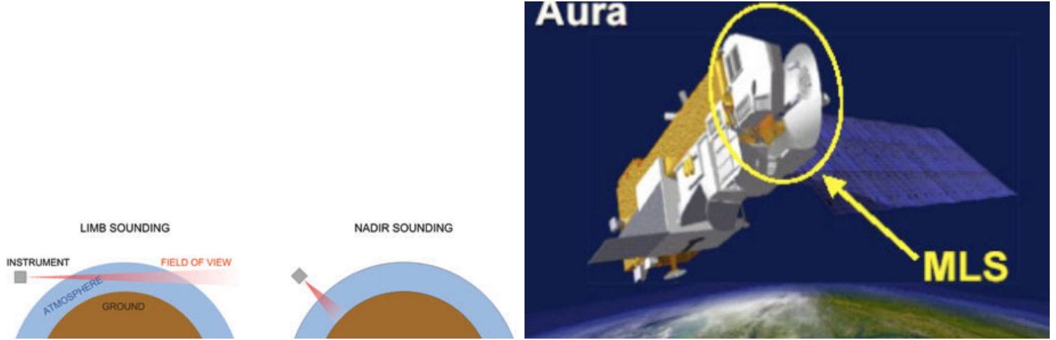
Figure 33: Limb and Nadir sounding (left) and the System Microwave limb sounder (MLS, right)
