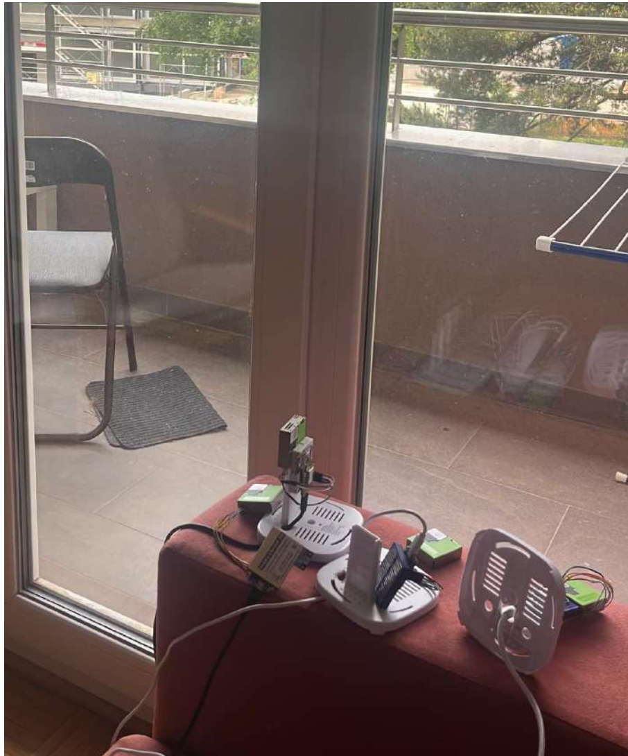
Figure 23: Illustration of the collocated low-cost sensors
