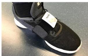
Fig. 1: foot-worn inertial sensor
